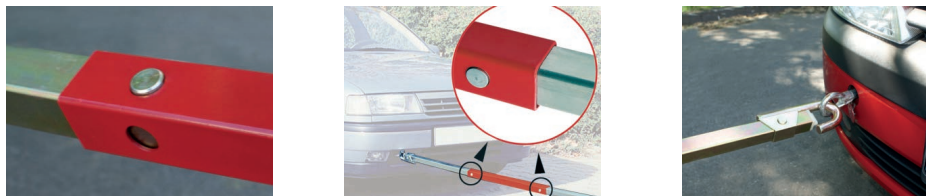
Figure 1: Connecting the vehicles
