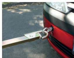
Figure 1: Connecting the vehicles
