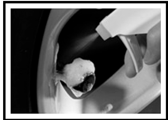
6. Check for any leakage with soap and water
