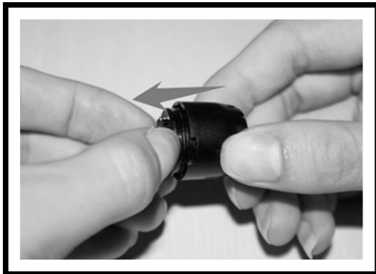
5. Pull apart the sensor housing with the help your fingernail
