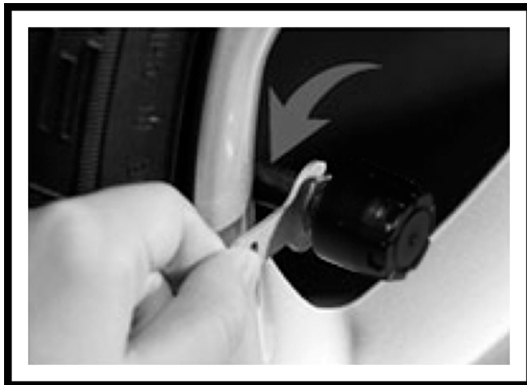
4. Use the delivered nut wrench to tighten the hex nut to the sensor
