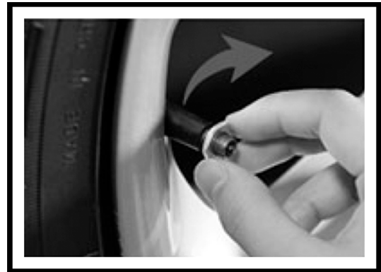
2. Put on the delivered hex nut
