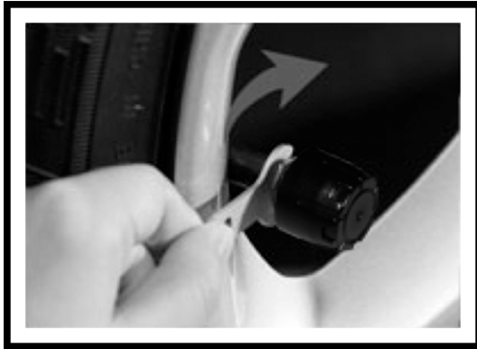
1. Release the hex nut with the delivered wrench
