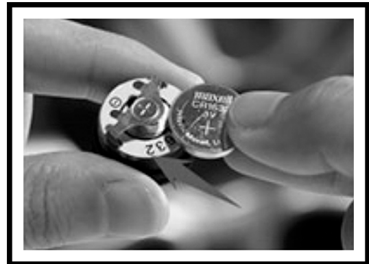
6. Exchange the CR1632 button cell battery (+ plus facing upwards)
