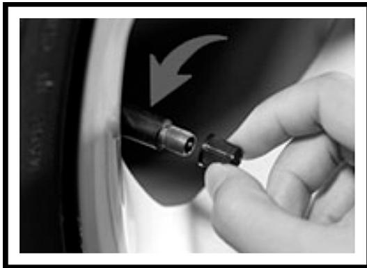
1. Remove the dust cover of the valve
