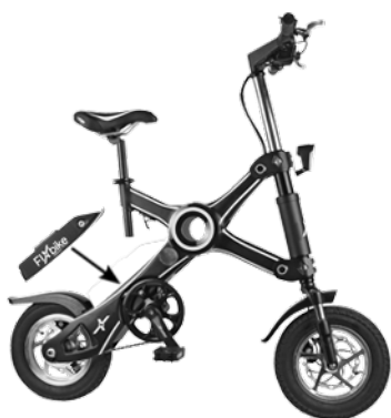
Image 5: Inserting the battery
