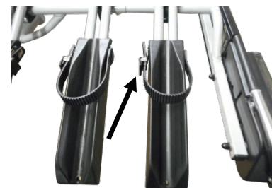
Figure 8: Installation position of closures
